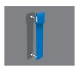
STEP 3 Firmly adhere the tape to the test surface with the quarters at the top. Allow the tape to support the quarters.
